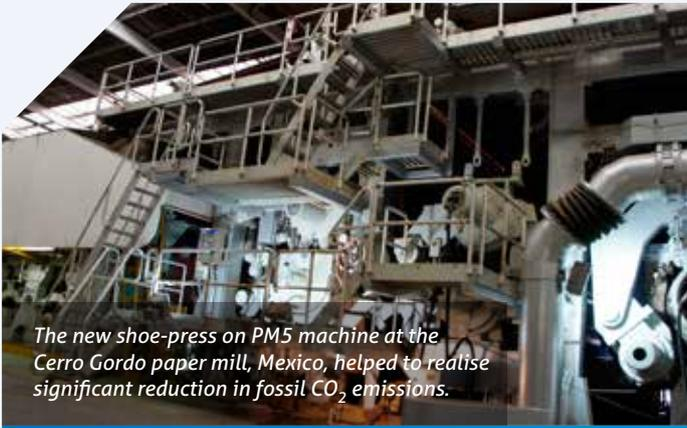
*The new shoe-press on PM5 machine at the Cerro Gordo paper mill, Mexico, helped to realise significant reduction in fossil CO<sub>2</sub> emissions.*
